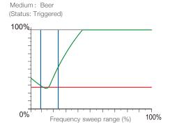
Sometimes, the Dk value of the two media may be the same. So how to separate? Setting two independent switch points does not help (two blue lines).
